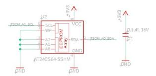
Connect A0-A2 to GND in order to be compatible with 24CW640T EEPROM  $_{\star} addr$  = 0X 50
