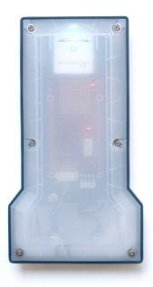
The Monitor One is an off-the-shelf complete gateway design, like the Tracker One. The Monitor One is in a larger IP67 waterproof enclosure with room inside for an expansion card and additional connectors, allowing it to be used in more custom scenarios than the Tracker One.
