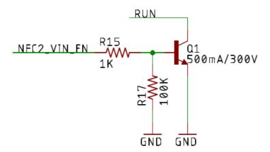
By disconnecting the VIN power supply, it reduces the current used by the VIN and PMIC voltage regulators. The Monitor One can still be powered by its internal LiPo battery. This is particularly advantageous if the Monitor One is in sleep mode while VIN is disconnected as the power supply loss will be large compared to the very low sleep current in this scenario.
