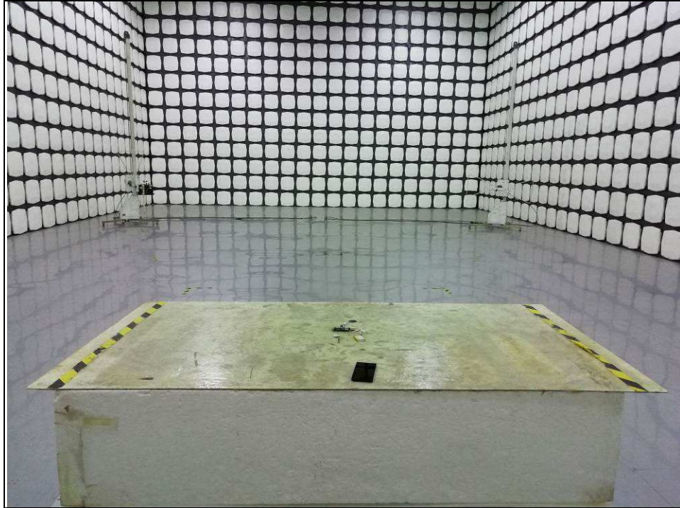
RADIATED EMISSION TEST (30MHz-1GHz)
