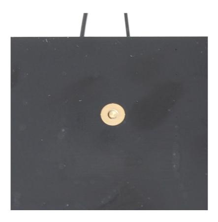
• As these parts may be difficult to source, for prototyping you can use a M3 screw, 6.5mm long, and a M3 nut. Use a 3mm non-plated hole in the base board. Note that a screw is required, as the M.2 connector does not self-lock.
