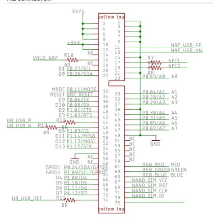
Note: The labels for CTS and RTS are reversed in this schematic.
