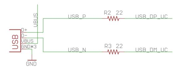
The USB data lines are terminated with 22 Ohm resistors. These data pins are also exposed via small through holes next to the USB connector and are labeled D+ and D-. The VBUS (+5VDC VCC of the USB port) is fed to the PMIC via a 3Amp Schottky diode (\$\sigma 53P3\$). The VBUS pin is also available via the unpopulated header hole on the top-right side of the E series.
