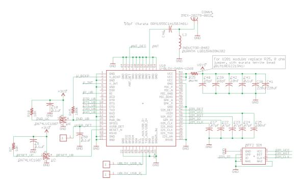
The u-blox cellular module talks to the microcontroller over a full-duplex USART interface using a standard set of AT commands. The MFF2 embedded SIM chip is directly connected to the u-blox module.
