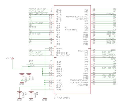
The E series uses ST Microelectronics's STM32F205RGT6 ARM Cortex M3 microcontroller running at 120MHz.
