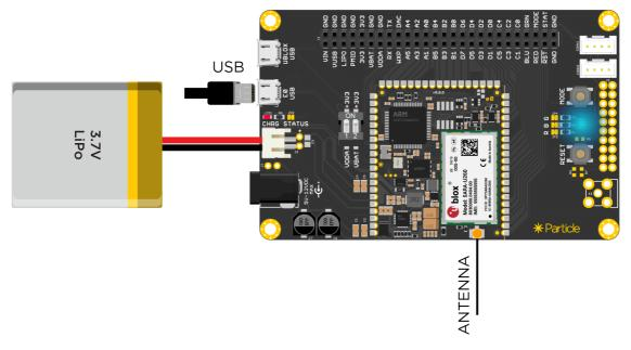
Plug the antenna into the uFL connector. Remember never to power up the Electron or this board without the antenna being connected. There is potential to damage the transmitter of the u-blox module if no antenna is connected.
