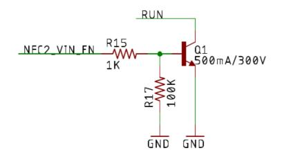
By disconnecting the VIN power supply, it reduces the current used by the VIN and PMIC voltage regulators. The Monitor One can still be powered by its internal LiPo battery. This is particularly advantageous if the Monitor One is in sleep mode while VIN is disconnected as the power supply loss will be large compared to the very low sleep current in this scenario.
