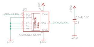
Connect A0-A2 to GND in order to be compatible with 24CW640T EEPROM , addr = 0X 50  $\,$
