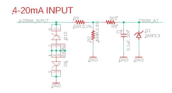
The A7 pin measures the voltage across R2, which is 100  $\Omega$ .
