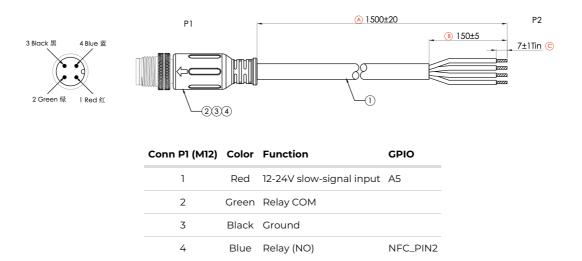
See M12 connector ratings below for voltage and current limits for this connector.
