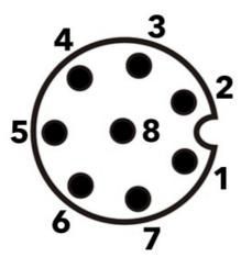
Looking at the pins on the end of the connector on the cable
