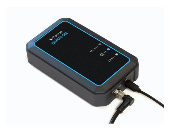
Particle gateway device like the Monitor One and Tracker One are designed to be used off-the-shelf to interface to other devices and sensors using standard protocols such as CAN bus, I2C, and serial.
