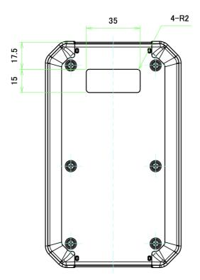
Maximum Carrier Board Dimensions (mm):
