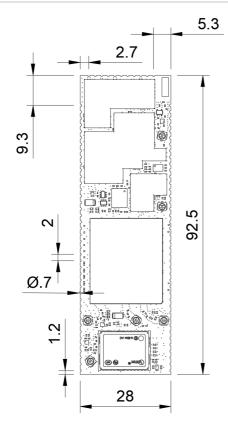
Dimensions are in millimeters.
