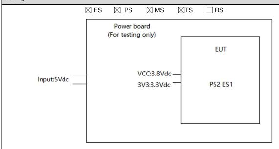
ES1:All parts within EUT; PS2: All parts within EUT;
