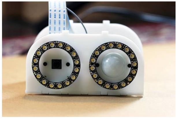
4. Attach the top plate and secure it to the bottom using M3 screws
