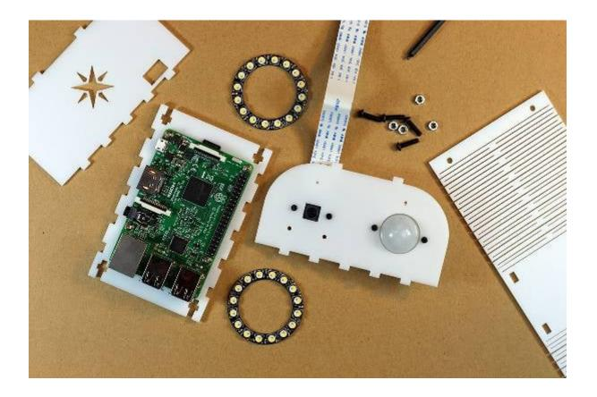
1. Attach the Pi to the base plate using M2.5 screws and nuts
