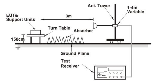
For the actual test configuration, please refer to the attached file (Test Setup Photo). **CONDUCTED POWER MEASUREMENT:**
