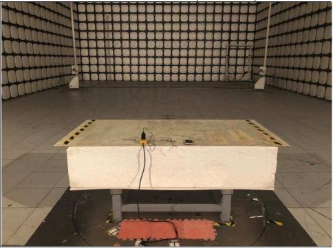
RADIATED EMISSION TEST (Above 1GHz)
