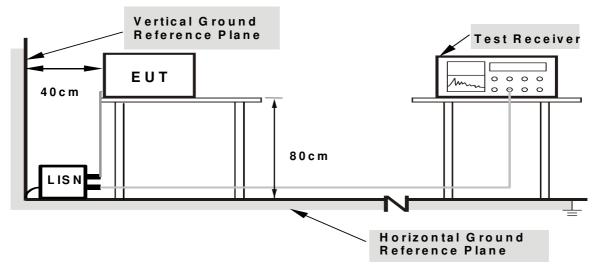
Note: 1.Support units were connected to second LISN. 2.Both of LISNs (AMN) are 80cm from EUT and at least 80cm from other units and other metal planes support units.
