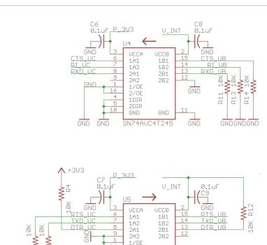
Since u-blox module's communication interface operates at 1.8VDC, while the STM32F205RGT6 microcontroller operates at 3.3VDC, we need voltage translators in-between them. This is achieved with two <u>SN74AVC4T245</u> non-inverting buffers. The default state of the USART pins is set with the help of pull-up and pull-down resistors, and the unused input pins are tied to GND.
