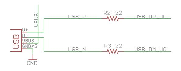
The USB data lines are terminated with 22 Ohm resistors. These data pins are also exposed via small through holes next to the USB connector and are labeled D+ and D-. The VBUS (+5VDC VCC of the USB port) is fed to the PMIC via a 3Amp Schottky diode (<u>SS3P3</u>). The VBUS pin is also available via the unpopulated header hole on the top-right side of the E series.
