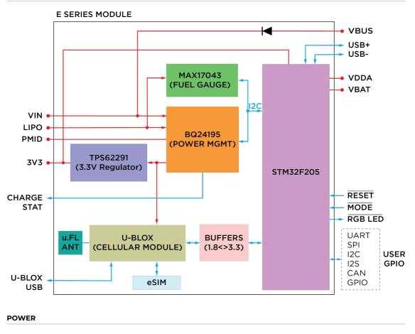
The E series can be powered via the VIN (3.88V-12VDC) pin, over USB, or a LiPo battery.
