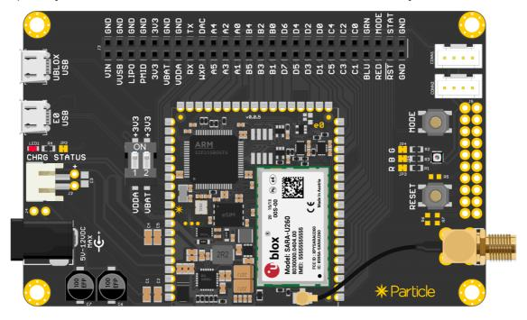
There are two 4-pin connectors available for you to plug in Grove compatible sensors. CONN1 exposes two analog pins (A0 and A1) while CONN2 exposes the I2C pins (D0 and D1).
