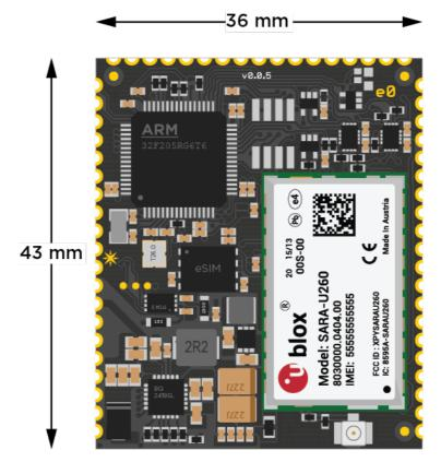
This diagram indicates only the dimensions; the components on the module will be different.
