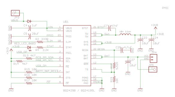
The Electron uses TI's BQ24195 as the power management and charging unit. This PMIC intelligently sources power from either the VIN pin, the USB port and/or the LiPo battery. When all
