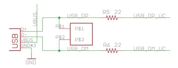
The USB data lines are terminated with 22 Ohm resistors. These data pins are also exposed via small through holes next to the USB connector and are labeled D+ and D-. The VBUS (+5VDC VCC of the USB port) is fed to the PMIC via a 3Amp Schottky diode (\$53P3). The VBUS pin is also available via the unpopulated header hole on the top-right side of the Electron.
