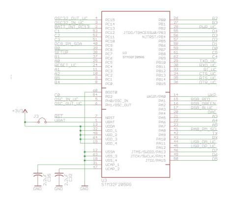
The Electron uses ST Microelectronics's STM32F205RGT6 ARM Cortex M3 microcontroller running at 120MHz.
