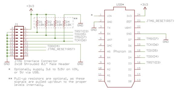
**Note:** This interface is not supported by the P0 module and cannot be used.
