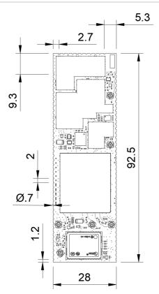
Dimensions are in millimeters.
