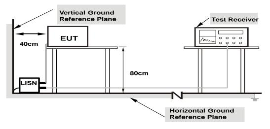
Note: 1.Support units were connected to second LISN. 2.Both of LISNs (AMN) are 80 cm from EUT and at least 80 cm from other units and other metal planes
