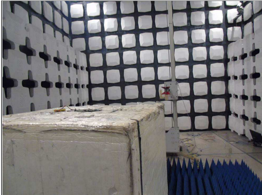
SPURIOUS EMISSION TEST ABOVE 1GHz
