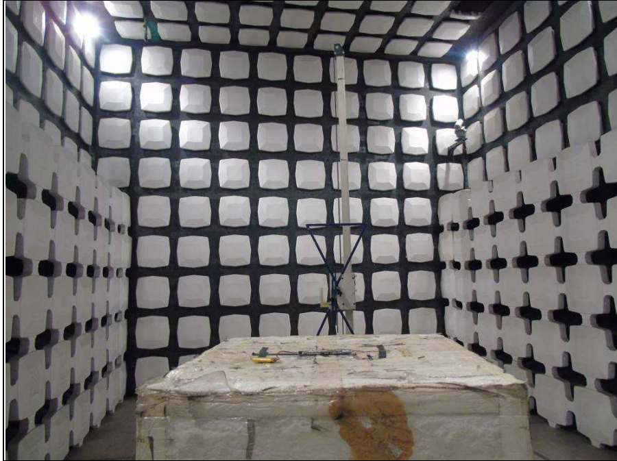
SPURIOUS EMISSION TEST BELOW 1GHz
