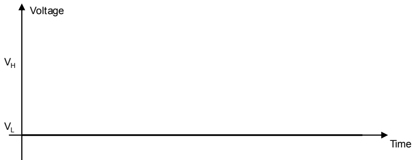
Figure 4: GPIO pin progress for no service
