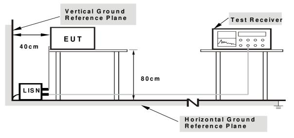
Note: 1.Support units were connected to second LISN. 2.Both of LISNs (AMN) are 80cm from EUT and at least 80cm from other units and other metal planes support units.
